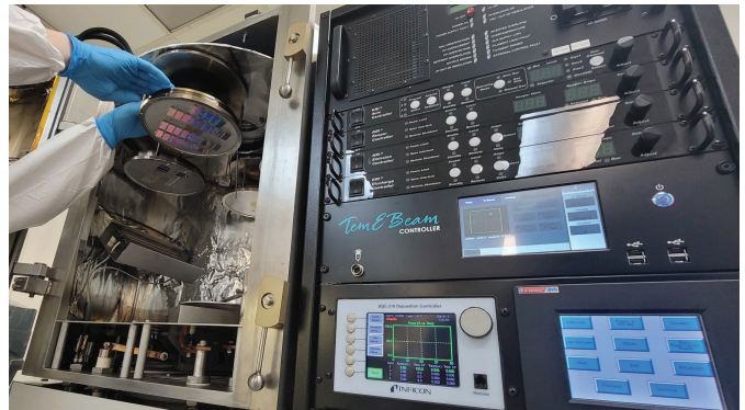
Fig 3: SSI Ion Assisted E-beam Coating System
